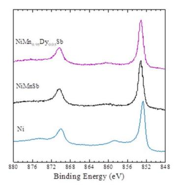
Fig. 3. Ni 2p XPS spectra of Ni, NiMnSb and Mn<sub>0.95</sub>Dy<sub>0.05</sub>NiSb alloys
