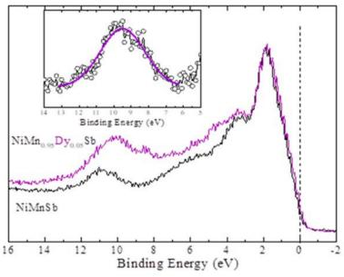
Fig. 5. XPS valence band spectra of NiMnSb and  $Mn_{0.95}Dy_{0.05}NiSb$  alloys
