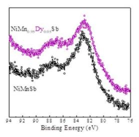
Fig. 2. XPS Mn 3s core level spectra of Mn<sub>0.95</sub>Dy<sub>0.05</sub>NiSb and MnNiSb
