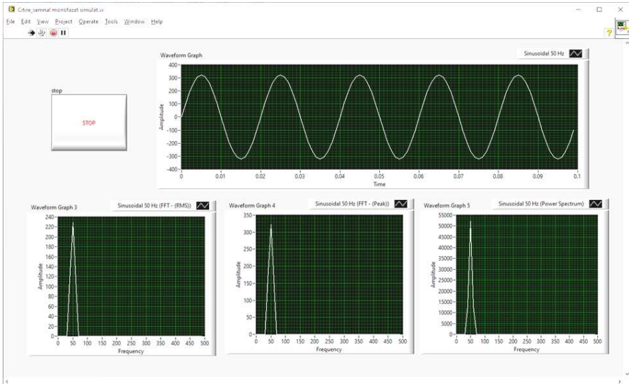
Figure 5. Simulation results for 50Hz frequency and 325 amplitude signal
