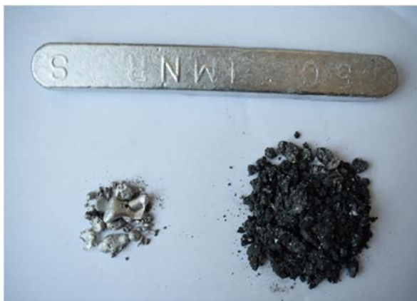
Fig. 6. Aluminium metallic ingot and slags obtained on the melting process of the aluminium beverage cans
