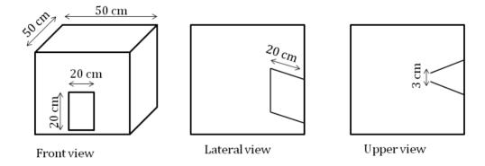
Figure 2. The design of Potter's traps.
