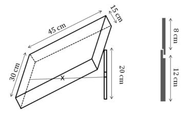
Figure 3. The designee of automatic fall traps.
