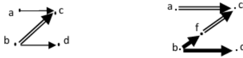
FIGURE 8. “Z” configuration, his corresponding transformation in AoN graph and the partition of the complete bipartite.
