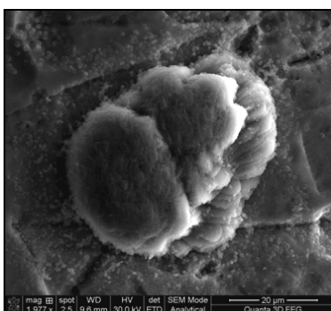
Figure 5b. Manganese dioxide germination on Ti–after S2 step; Electrolyte: 1M H 2 SO 4 + 6g/L Mn 2+ , pH≈-0.5, sweep rate 2mVs -1
