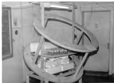
Picture 1. Helmholtz Coil System
