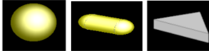
Figure 1. Example of nanoparticles shapes (sphere, rod, and prism) we study in this work.
