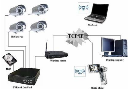
FIGURE 1. Video surveillance/monitoring system
