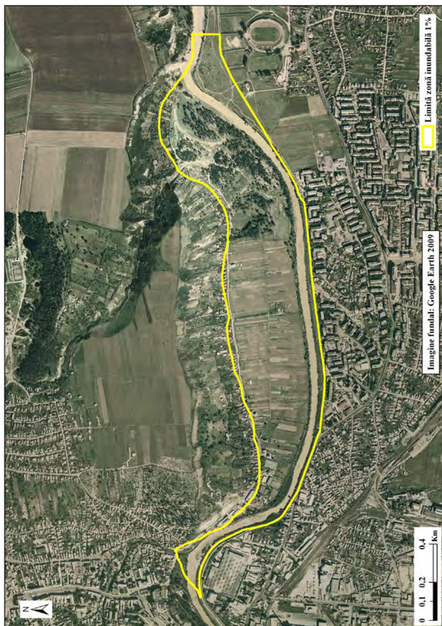
Fig. 2. The flooded area related to the non-exceedence probability of 1% on the Aries Valley at Turda
