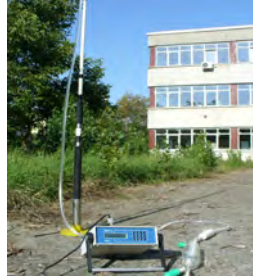
Fig. 2. The NDIR, used for the CO 2 determination.
