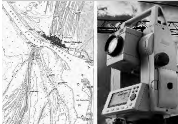
Fig. 1(a) and (b) . Topo-hydrographic map from 1965 (a) and the total station Leica TPS 407 (b) used for the development of the land section of the topo-bathymetric model in the area of study
