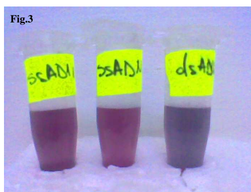
Fig. 3. Photographic image of gold colloid mixtures with (from left to right): ssDNA, ssDNAc and dsDNA in which NaCl solution was introduced.
