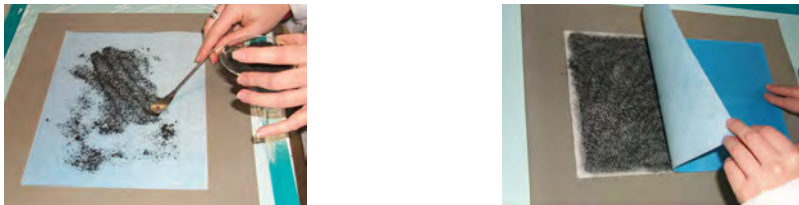
Figure 4. Manual doping of impregnated laminates.
