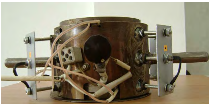
Figure 1. The plates fabrication mould.
