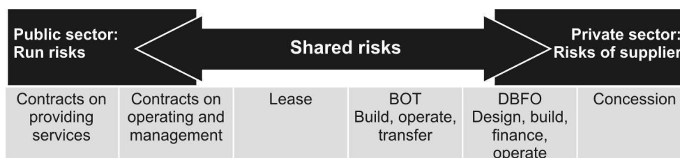
Chart 2: Allocation of risks in the PPP projects depending on a type of a project
