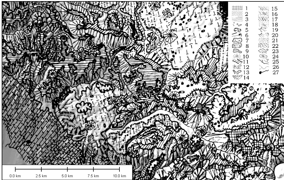
Fig. 2. Geomorphological map of the Pădurea Craiului (1.Upper erosion level (800-1000m); 2.Medium erosion level (600-650m); 3.Lower erosion level (400-450m); 4. Dolina; 5. Uvala; 6. Pit-ponor; 7. Karst depression, 8. Karst plateau; 9.Karst plain, 10. Hum; 11. Gorges, 12. Gully erosion; 13. Torrents; 14.Alluvial cone; 15. Lower terrace; 16. 7-15 and 20-25m terrace 17. 55-60m terasse; 18. 75-90m terasse; 19. Karst slope; 20. Clay slope; 21. Glacis; 22.Piedmont alluvial plain; 23. Erosion depression (Roşia), 24. Inselberg; 25. Rivers; 26. Temporary rivers ; 27. Sources.
