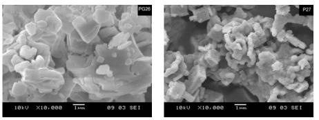
Fig. 5. SEM images of precursor (left) and phosphor (right)
