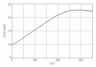
Fig. 1. A typical curve for  $O_2$  evolution, recorded with the Clark sensor in the reaction mixture pH=7 at  $20^{\circ}$ C
