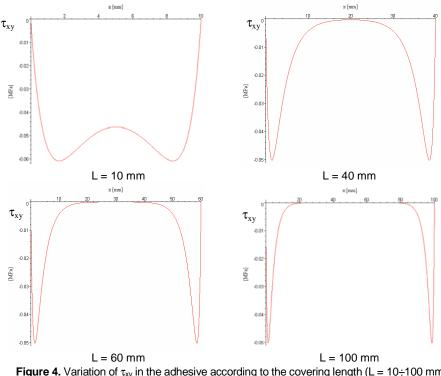
$\label{eq:Figure 4. Variation of $\tau_{xy}$ in the adhesive according to the covering length (L = 10÷100 mm)$$ and $F = 1 N/mm$, for a VE $\pm45°AV 119-VE $\pm45° assembly.$}$
