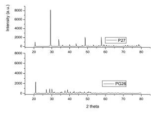
Fig. 2. XRD patterns for precursor (PG26) and phosphor (P27) prepared at 1200°C
