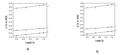
**Fig. 7.** Dependence of the formal standard potentials on the Li<sup>+</sup> concentration for:  $[Bu_4N]_{10}H_2[(CeO)_3(PW_9O_{34})_2]$  (a) and  $[Bu_4N]_{10}H_2[(CeO)_3(AsW_9O_{34})_2]$  (b) (v= 100 mV s<sup>-1</sup>).
