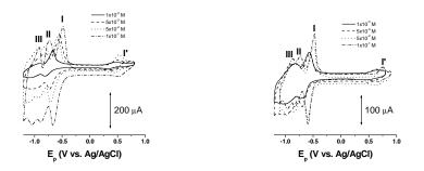
Fig. 6. Cyclic voltammograms of  $[Bu_4N]_{10}H_2[(CeO)_3(PW_9O_{34})_2]$  (a) and  $[Bu_4N]_{10}H_2[(CeO)_3(AsW_9O_{34})_2]$  (b) at different concentrations of LiClO<sub>4</sub> (0.1 M [Bu<sub>4</sub>N]ClO<sub>4</sub> in acetonitrile, v= 100 mV s<sup>-1</sup>).
