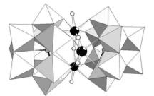
**Fig.1.** The polyhedral representation of the sandwich polyoxotungstocerates (WO<sub>6</sub> white octahedral; Ce – black spheres; P – grey spheres; O- white spheres).
