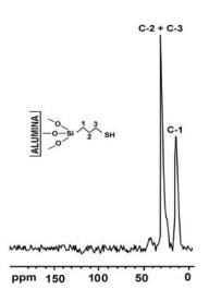
Figure 5. <sup>13</sup>C-CP/MAS NMR spectrum of alumina-SH
