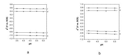
Fig. 4. Dependence of the formal standard potentials on the pH for:  $K_{10}H_2[(CeO)_3(OH_2)_2(PW_9O_{34})_2] \cdot 18H_2O$  (a) and  $K_{10}H_2[(CeO)_3(OH_2)_2(AsW_9O_{34})_2] \cdot 21H_2O$  (b) (v= 100 mV s<sup>-1</sup>).
