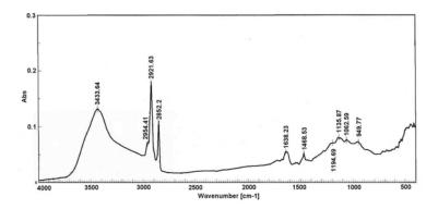
FIGURE 3. Difference FTIR spectrum of alumina-C18 and alumina
