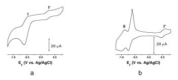
Fig. 5. Cyclic voltammograms of  $[Bu_4N]_{10}H_2[(CeO)_3(PW_9O_{34})_2]$  (a) and  $[Bu_4N]_{10}H_2[(CeO)_3(AsW_9O_{34})_2]$  (b) (0.1 M  $[Bu_4N]CIO_4$  in acetonitrile, v= 100 mV s<sup>-1</sup>).
