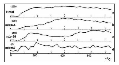
**Figure 7.** Intensity of characteristic ions *versus* temperature for alumina-C18: **a**) I total, **b**)  $m/z = 44 [CO_2]^{\dagger}$ , **c**)  $m/z = 36 [HCI]^{\dagger}$  ion, **d**) m/z = 57 (organic part) ion
