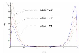
Figure 6. Variation of the shear stress  $(-\tau_{xy})$  according to relative rigidity.
