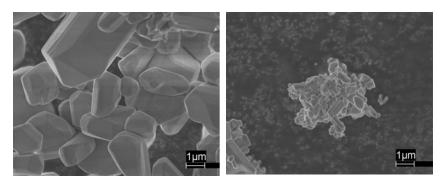
Fig. 3. SEM images of  $YTa_{0,85}Nb_{0.15}O_4$  samples prepared with different fluxes: T7 -  $Li_2SO_4$  (left) and T9 -  $Na_2SO_4$  (right)
