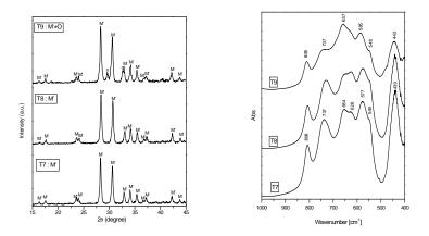
Fig. 2. XRD patterns (left) and FT-IR (right) spectra of YTa<sub>0.85</sub>Nb<sub>0.15</sub>O<sub>4</sub> samples prepared with different fluxes,T7= Li<sub>2</sub>SO<sub>4</sub>]; T8= Li<sub>2</sub>SO<sub>4</sub>+Na<sub>2</sub>SO<sub>4</sub>; T9= Na<sub>2</sub>SO<sub>4</sub> (M'=M'-YTaO<sub>4</sub> and O= orthorhombic Y<sub>3</sub>TaO<sub>7</sub> structures)
