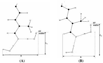
**Fig.5.** The shape of the lower part of the APO-molecule and the size of its hydrated polar head group for a vertical orientation of the molecular axis – 1<sup>st</sup> inertial axis (A) and for an angle of 20° to the vertical (B)
