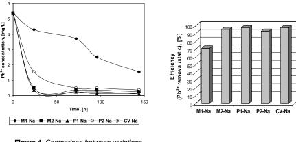
**Figure 4.** Comparison between variations of *Pb*<sup>2+</sup> concentration (in the synthetic wastewater) in time for all zeolitic volcanic tuffs studied, in -Na form and static regime.
