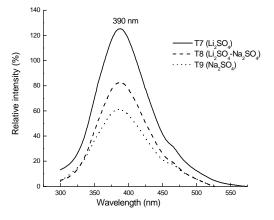
**Fig. 1.** Emission spectra of  $YTa_{0.85}Nb_{0.15}O_4$  samples ( $\lambda_{exc}$ = 254 nm)
