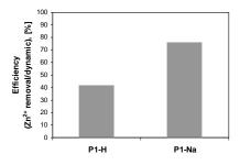
Figure 1. Ionic exchange efficiency for zinc removal on P1 zeolitic volcanic tuff subjected to acid (P1-H) and acid-alkaline treatment (P1-Na)
