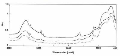
Figure 2. FTIR spectra of: a, alumina-C18; b, alumina-SH, c, alumina
