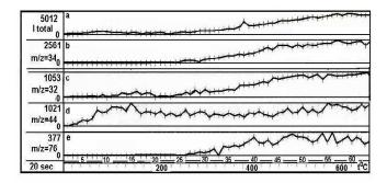
**FIGURE 9.** Intensity of characteristic ions *versus* temperature for alumina-SH: **a**) I total, **b**)  $m/z = 34 [SH_2]^+$  ion, **c**)  $m/z = 32 [CH_3-OH]^+$  ion, **d**)  $m/z = 44 [CO_2]^+$  ion, **e**)  $m/z = 76 [C_3H_8S]^+$  ion
