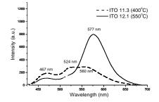
Fig. 4. Emission spectra of some ZnS: Cu, Mn films deposited onto ITO layer
