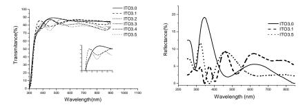
Fig. 1. Transmission spectra of some ZnS/ITO/glass heterostructures
