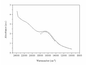
Fig.4. The visible electronic spectrum of the Cr<sup>JII</sup>AsW<sub>3</sub> complex in 5x10<sup>-3</sup> mol·l<sup>-1</sup> aqueous solution. The Gaussian components are represented with dashed lines.
