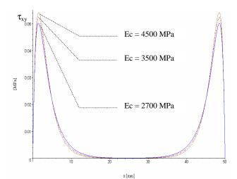
Figure 5. Variation of the shear stress  $(-\tau_{xy})$  in the adhesive according to the elastic module of the adhesive.
