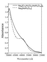
Fig. 3. UV spectra of the sodium salts of  $Cr^{III}AsW_9$  (solid) and  $AsW_9$  (dotted) obtained in  $5x10^{-5}$  mol·l<sup>-1</sup> aqueous solution.
