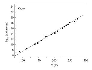
**Fig. 5.** Variation of reciprocal molar susceptibility of the  $Cr^{III}AsW_9$  complex with respect to temperature. Solid line represents the best fit of the experimental data with a Curie-Weiss behavior.
