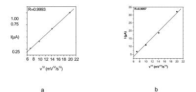
Fig. 3. Dependence of the cathodic peak I current on the scan rate for:  $K_{10}H_2[(CeO)_3(OH_2)_2(PW_9O_{34})_2] \cdot 18H_2O$  (a) and  $K_{10}H_2[(CeO)_3(OH_2)_2(AsW_9O_{34})_2] \cdot 21H_2O$  (b) (pH=4.0).
