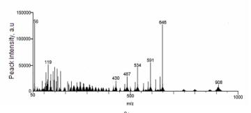
Fig. 2. Mass spectrum of the 1:1 UO<sub>2</sub><sup>2+</sup>:p-tert-butylcalix[4]arene complex.
