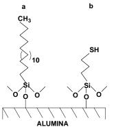
Figure 1. Chemically modified alumina: a, alumina-C18; b, alumina-SH
