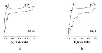
Fig. 2. Cyclic voltammograms of  $K_{10}H_2[(CeO)_3(OH_2)_2(PW_9O_{34})_2]$ ·18H<sub>2</sub>O (a) and  $K_{10}H_2[(CeO)_3(OH_2)_2(AsW_9O_{34})_2]$ ·21H<sub>2</sub>O (b) recorded in aqueous solutions (pH= 4.0, v= 50 mV s<sup>-1</sup>).
