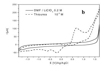
Figure 2. CVs for the oxidation of ligand and (TU) on GC electrode in DMF/ 0.2 M LiClO<sub>4</sub> for :  $a - oxidation of 10^{-3} M (TSCSA)$  $b - oxidation of 10^{-3} M (TU)$
