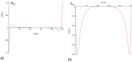
**Figure 3.** Distribution of the stresses in the adhesive of a VE  $\pm$ 45°AV 119-VE  $\pm$ 45°assembly for F = 1 N/mm. a) the peeling stress ( $\sigma_{vv}$ ), b) the shear stress ( $\tau_{xv}$ ).
