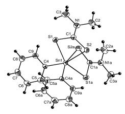
Figure 4. ORTEP representation at 30% probability and atom numbering scheme for Ph<sub>2</sub>Sn(S<sub>2</sub>CNMe<sub>2</sub>)<sub>2</sub> (4).
