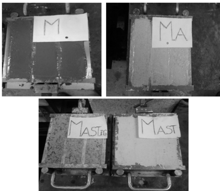
Fig. 3. Mixtures of the four composite molded into standardized moulds (40x40x160 mm)
