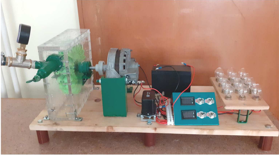
Figure 6. The laboratory micro hydroelectric power plant.
