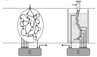
**Figure 2**: Analogy between a reservoir computing system and the octopus robotic arm modelled as a physical reservoir computing system by Nakajima, Hauser, Li and Pfeifer. The units of the physical reservoir are sensors coupled through a soft silicone material. See: K. Nakajima, H. Hauser, T. Li and R. Pfeifer, *Information Processing*, cit., p. 3.
