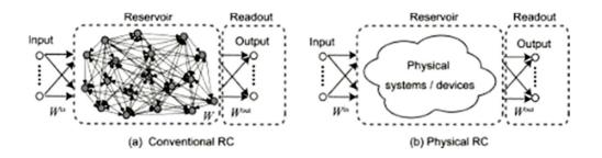
**Figure 1**: Conventional and physical approaches to reservoir computing systems. (a) In conventional reservoir systems the reservoir is an artificial recursive neural network. (b) In physical reservoir systems the reservoir describes a natural system or a device. See: Tanaka et al., *Recent Advances*, cit., p. 3.
