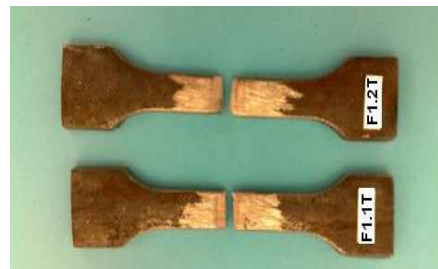
Figure 4. Broken test piece F1T
