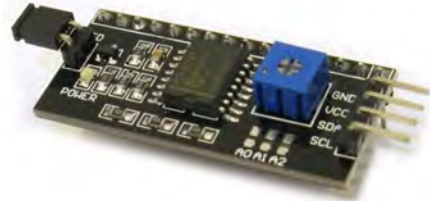
Figure 8. I2C LCD1602 adapter
