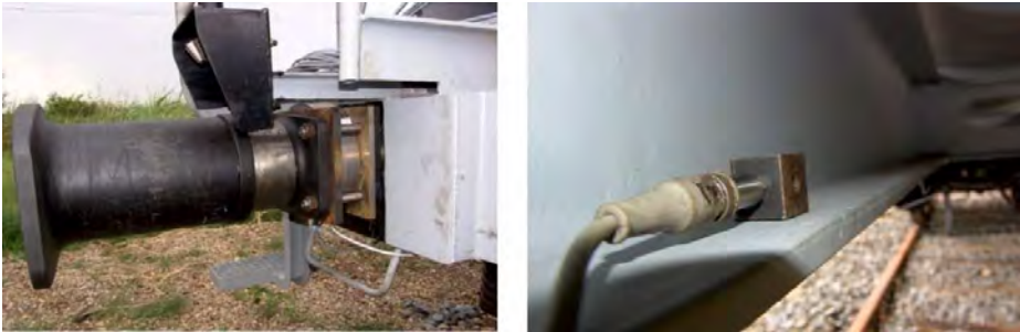
Figure 2. Force cell and accelerometer.
