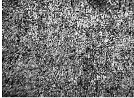
Figure 10. Sample F1T, WELD, Nital 2%, 100X
