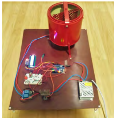
Figure 10. Model of centrifugal equipment with microprocessor for bee honey extract made
