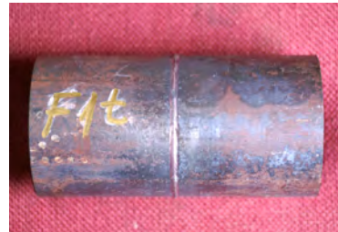
Figure 2. F1T butt welded sample, heat treated.
