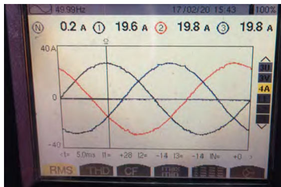
Figure 7. Current values on the three phases
