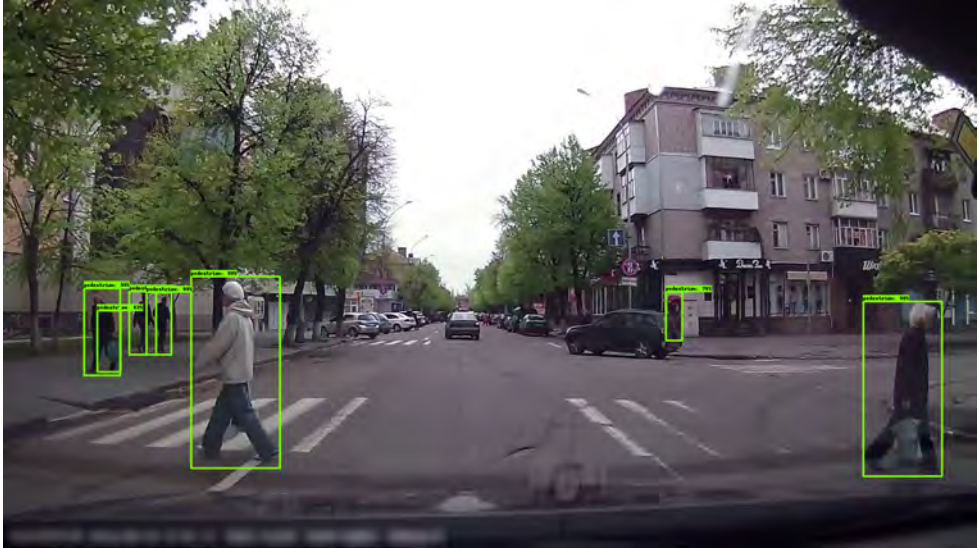
FIGURE 2. Pedestrian detection using the pedestrian tag for all pedestrians.
