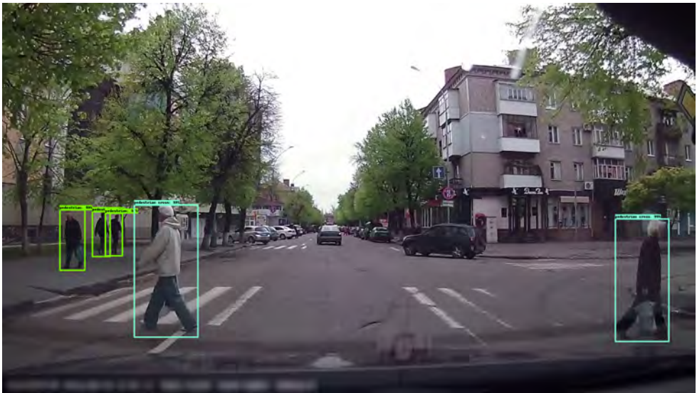
FIGURE 3. Pedestrian detection using multiple tags.
