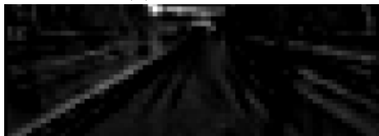
(B) The plotted values of neurons of a feature map situated after the second convolutional layer (and its activation) of the M2 model
